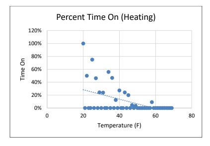
This data shows that during the heating season, the units ran 43% of the time at 0F and 6% of the time at 50F. Since these units are manually switched off until outdoor air temperatures reach about 20°F, the units are assumed to be off whenever the outdoor air temperature is below 50°F.
