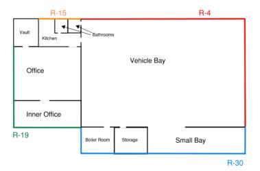
This measure looks into adding to the existing insulation to get all the walls in the Highway Garage up to an R-value of at least 30.
