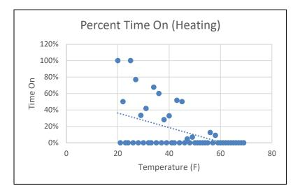
This data shows that during the heating season, the units ran 25% of the time at 0F and 17% of the time at 50F. Since these units are manually switched off until outdoor air temperatures reach about 20°F, the units are assumed to be off whenever the outdoor air temperature is below 50°F. These trends also lines up well with the usage in 2021.
