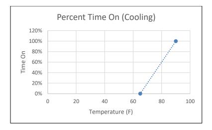
Due to the time of year of the study, C&S was unable to collect any meaningful data on these unit's cooling performance. Instead, a linear approximation was used for the cooling trends. It assumes that the unit is in cooling mode 100% of the time when the outdoor air temperature is 90°F or above, and 0% of the time when the outdoor air temperature is 65°F or below, and varies linearly between these two points.
