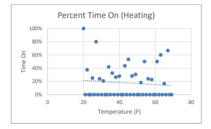
This data shows that during the heating season, the units ran 25% of the time at 0°F and 17% of the time at 50F. Since these units are manually switched off until outdoor air temperatures reach about 20°F, the units are assumed to be off whenever the outdoor air temperature is above 50°F. These trends also lines up well with the usage in 2021.
